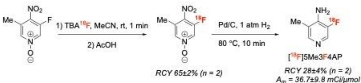
Scheme 1. Radiochemical synthesis of [ ^{18}\text{F} ]5Me3F4AP and radiochemical yield (RCY) based on radioHPLC.
