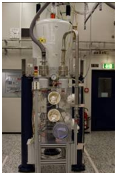
Photo of the 9.4 T Bruker NMR spectrometer with the radioactive glovebox available at JRC-ITU.
